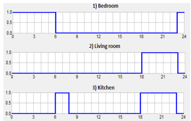
Fig. 6. Profile for the presence of the occupants on weekdays; 1 for fully occupied and 0 for absence.
