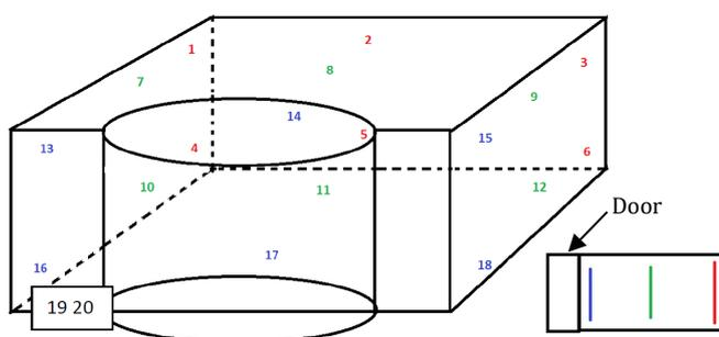
Figure 2. Positions of the thermocouples used for measurement.
